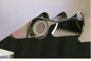
3-position slide lock limits trailer movement
